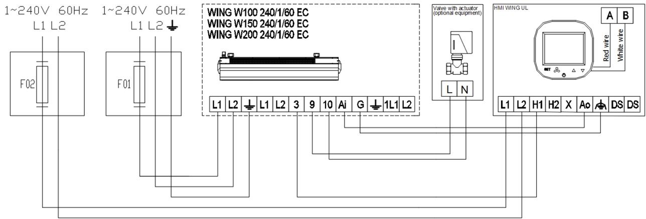
Figure 2 - WING W100/150/200 connections
