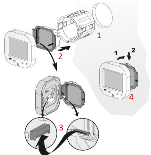
**CAUTION.** After all installation works, check if the flush mounting is properly done (the controller is fixed in the wall and is not loose).
